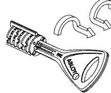
Fig. 4. The key can be turned back to the starting position and removed from the keyway. The combination is automatically scrambled by the two return bars. Unless this scrambling occurs, the key cannot be removed.
