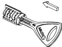
Fig. 1. The key meets little resistance when inserted into the keyway. There are no spring loaded parts to wear out.
