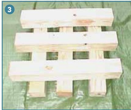
(3) 3 x 3 construction method uses three pieces per layer, each layer at right angles.
