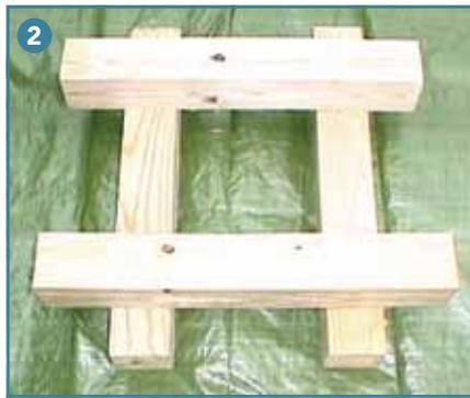
(2) 2 x 2 construction method of building a stack crib uses two pieces of cribbing per layer, each layer at right angles.
